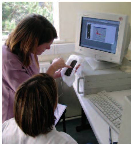
Figure 14 Jane Henderson advising a Cardiff University student on the use of digital x-radiography for the non-destructive investigation into the corrosion and technology of archaeological metals. Photo: David Watkinson
