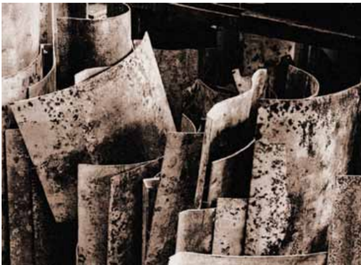
Victorian moulds for bending glass, John Bowden Ltd, 2006 Some of the moulds date back to the 1820s and would have required 20 men to lift them.
