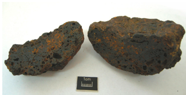
Figure 6 A cross section through a smithing hearth bottom (SHB) slag, which is a characteristically shaped lump of slag formed in a smith's hearth during iron smithing.
