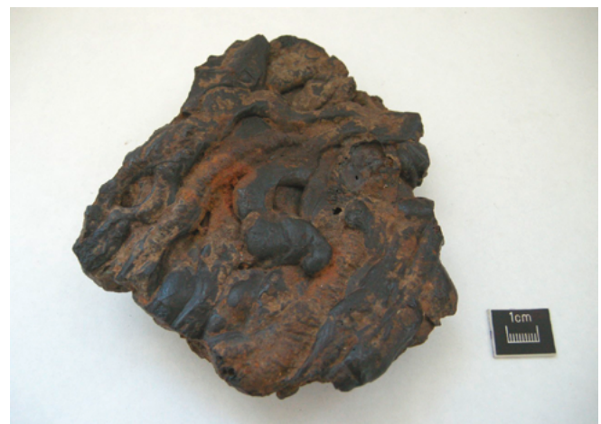
Figure 2 Tap Slag. This is waste from bloomery smelting, produced by a tapping furnace, and is easily identified by the flow patterns on the surface.
