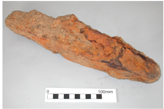
Figure 4 Iron billet. The iron blooms made by bloomery smelting had to be smithed before they could be used, to remove trapped slag and air. Then the iron was shaped into objects or a form of trade iron, such as a billet, ingot or bar. This is a billet of iron excavated from a Roman settlement at Westhawk Farm in Kent.
