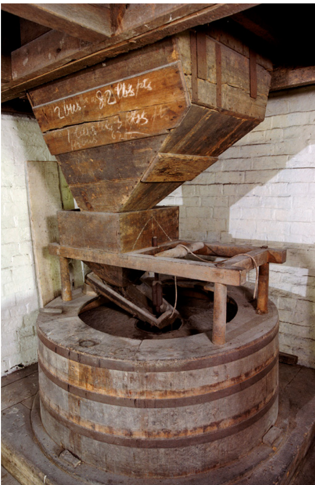
Figure 6 Interior of the former grind mill in the Hook Norton Brewery, Oxfordshire. The millstones, protected by a wooden 'tun', were turned by a shaft from below (see) and fed via the hopper from the floor above.
