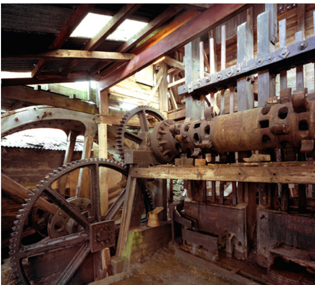
Figure 9 Interior view of waterwheel and stamps, Tolgus Tin Streaming Works, Cornwall. Here the waterwheel powered trip hammers. The trips can be seen on the horizontal drum to the right and the vertical hammers behind were used to crush ore.
