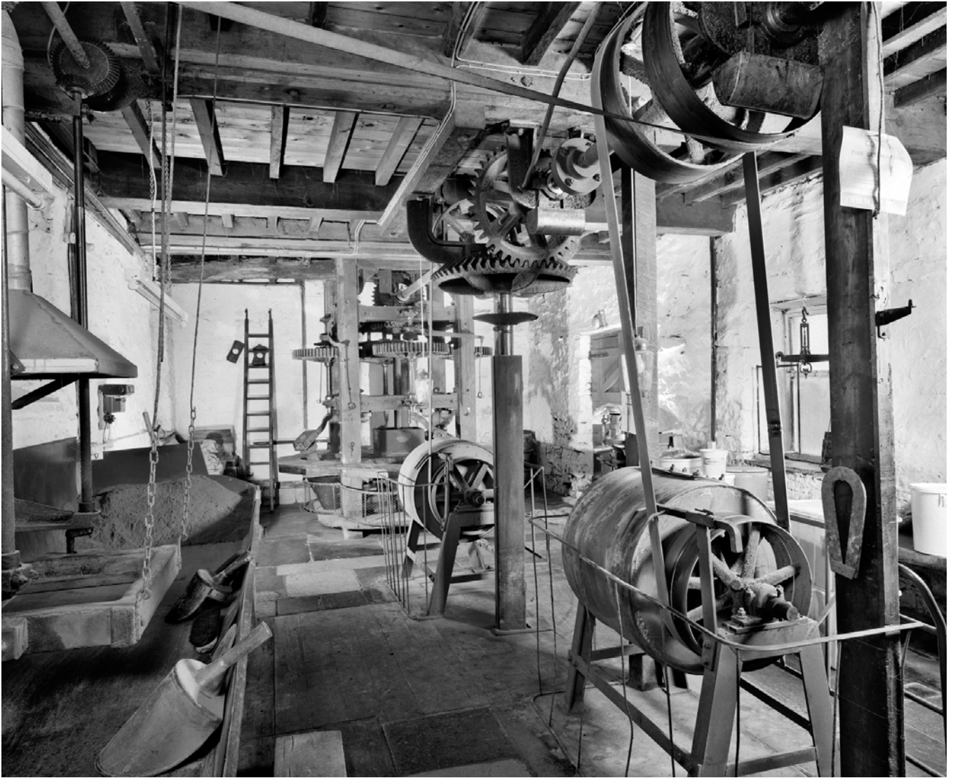
Figure 8 Helsington Snuff Mill, Cumbria. Waterwheels could power a wide range of machinery. A vertical shaft can be seen in the centre of the room running up, from gearing below, to horizontal overhead shafts, from which belts powered various machines.
