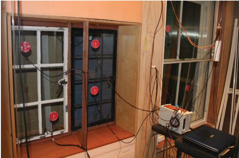
Testing the effectiveness of different improvements on historic steel, cast-iron and timber windows in the environmental chamber at Glasgow Caledonian University.
